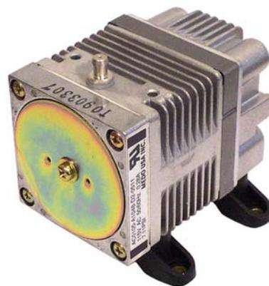
The Built-in “Whisper Quiet” Air Compressor provides an infinite and nearly silent supply of air for the FID, FID/DELCD, NPD, FPD, TID, or CCD detector. It mounts unobtrusively inside the 8610 or 310 GC chassis, and delivers unfiltered air to the detector.
